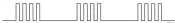
Figure 3.6 Pulse train signal on input A of Schmitt input NAMD (Test Point 323)
